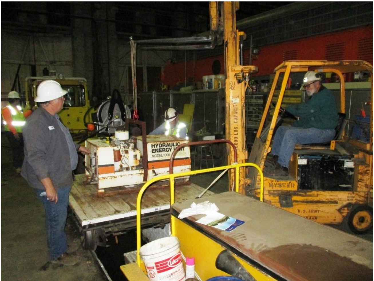
Alan lifts while Chris C. and Joe guide the new-used hydraulic power unit onto the flatcar
