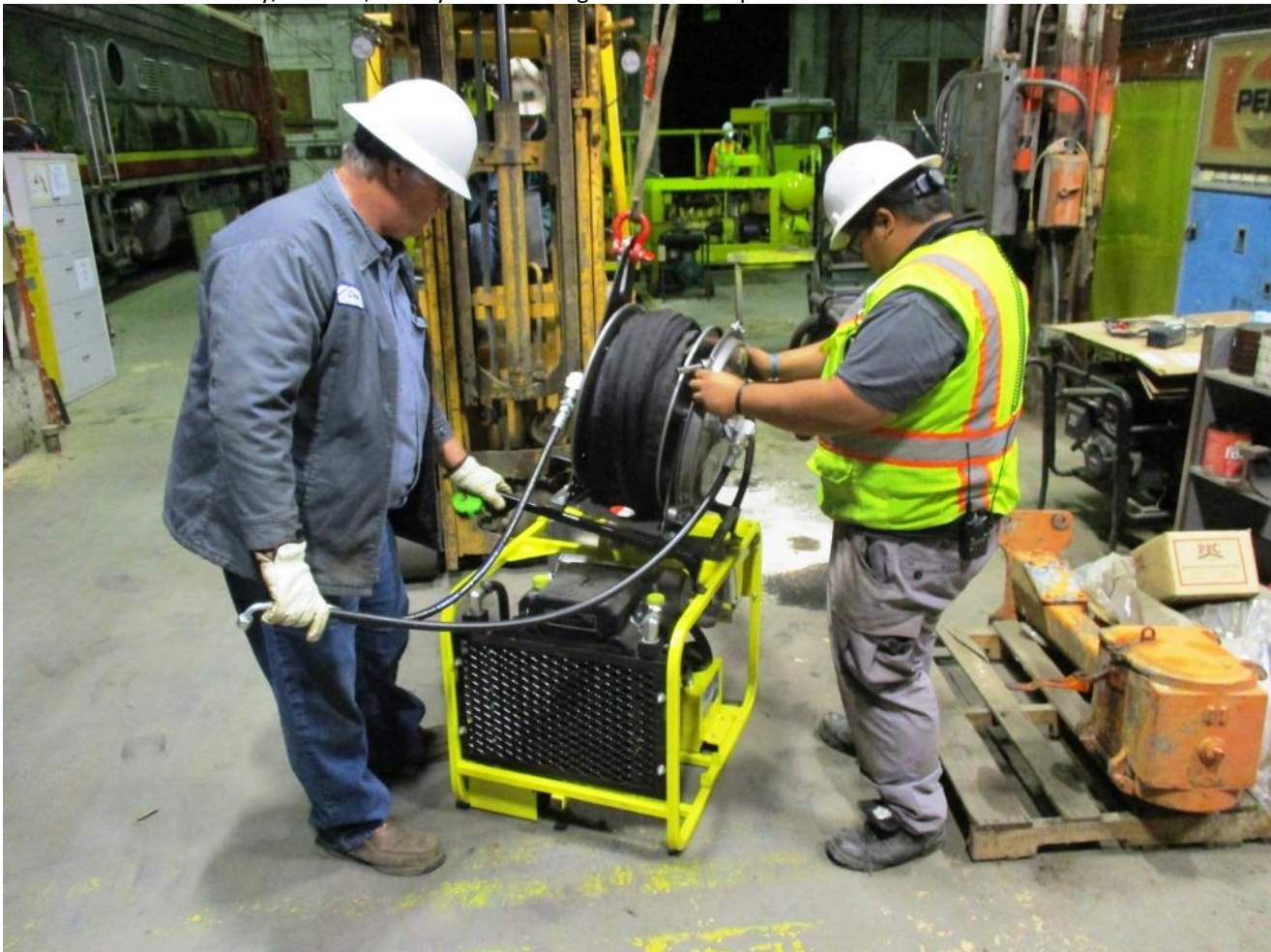
Chris C. and Anthony install the new hose-reel on the hydraulic power unit
